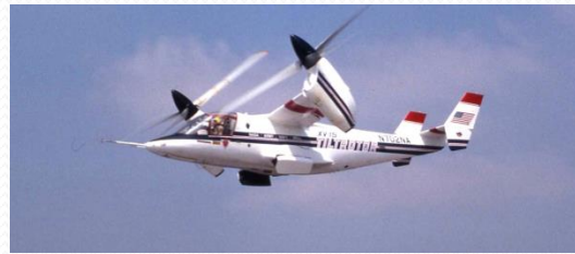
Transition (horizontal speed varies from zero to cruise speed)
