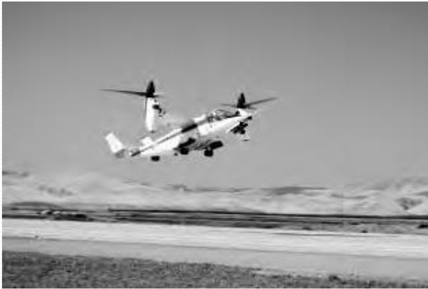
XV-15 during short takeoff performance test. (Ames Photograph AC82-0723-22)
